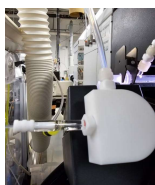
Figure 8. Nebulizer setup on Agilent 8900
