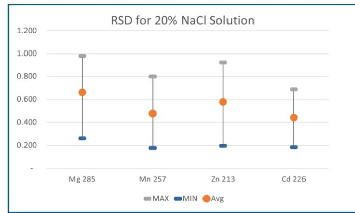
**Stability Test** - to demonstrate just how tough this nebulizer is, we ran a 20% NaCl solution through it for 6 hours. The results speak for themselves, virtually no drift, and no clogging!
